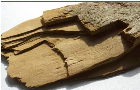
svn 42 Wet rot fungus – brown rot, leaf decomposition. Assessed as fungal damage. (Photo: Protox/Goritas)
