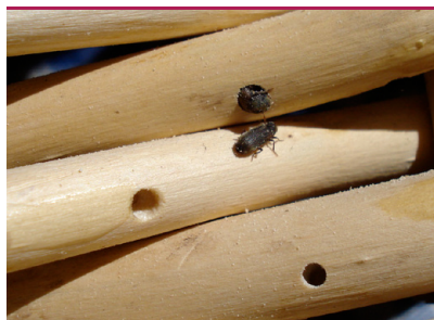
Common furniture beetles in wicker furniture in conservatory. (Photo: Protox)
