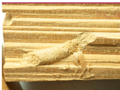
Wood wasp - larval stage with hard packed frass. (Photo: Prottox/Goritas)
