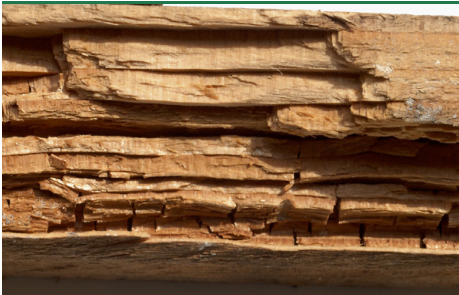
Serried crust fungus (Mine fungus) - decomposition. (Photo: Protox)
