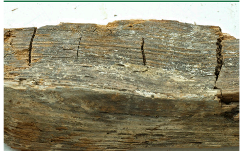
Dry rot fungus - old attack. Weak mycelial remains and clear transverse fissures. (Photo: Protox/Goritas)
