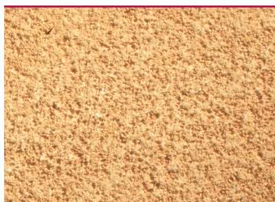
Common furniture beetles - frass. (Photo: Protox)
