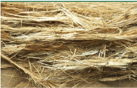
svn 52 White rot decomposition - unknown fungus. (Photo: Protox)
