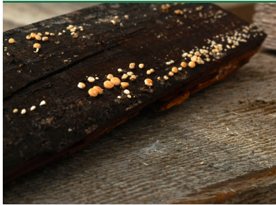
Ditiola radicata – fruiting bodies on exterior woodwork. (Photo: Protox)
