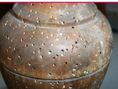
i 10 Common furniture beetles – exit holes in table legs. (Photo: Protox)
