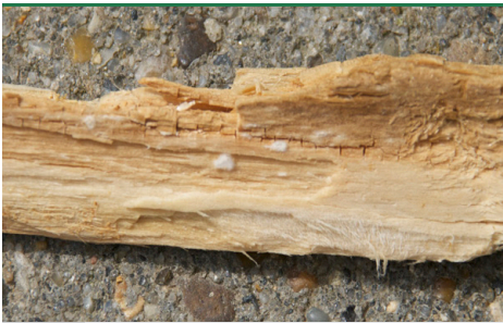
svn 39 Gilled polypore in outer covering. Note small tufts of surface mycelium on fracture surfaces (Photo: Protox)
