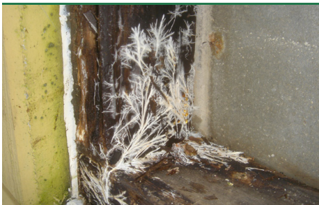
svn 38 Bark fungus – mycelium in frame wood. (Photo: Goritas)
