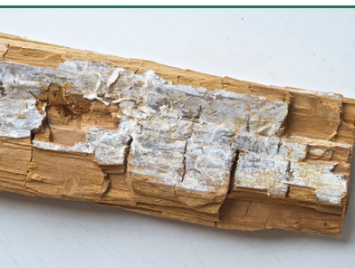
Mine fungus – decomposed wood (brown rot) and surface mycelium. (Photo: Protox/Goritas)
