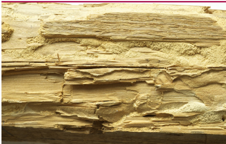
in 13 House longhorn beetle - exposed larval passages. (Photo: Protox/Goritas)
