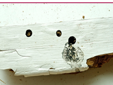
Red-brown Longhorn Beetle - exit holes 5-8 mm sharp-edged and round. (Photo: Protox/Goritas)
