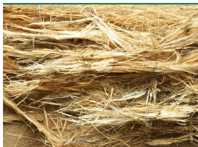
White rot - the fungus breaks down the lignin in the wood, leaving the cellulose threads. This frays the wood.
