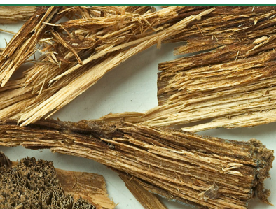
Cohesive aspen bracket fungus - decomposed wood (white rot) with a brownish coating. (Photo: Protox/Goritas)
